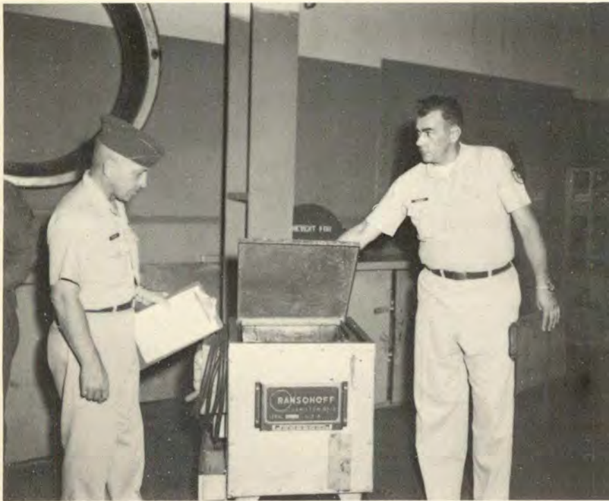
Inspecting the Hot Dip Direct Heating Tank
