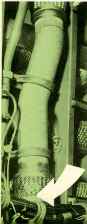
The appearance of the collapsed lower bellows and stretched upper unit could be a clue that the assembly is not installed correctly.
